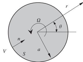
Fig. 3. A rotating cylinder in an infinite fluid.
