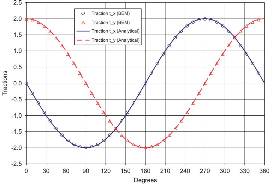
Fig. 4. Computed tractions on boundary  $S$  (with 40 elements).
