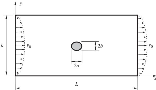
Fig. 8. Channel flow around a cylinder.
