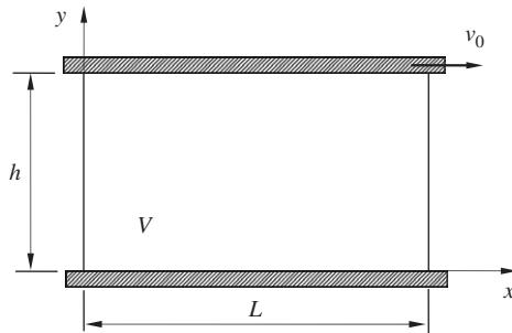
Fig. 7. Shear flow between two parallel plates.
