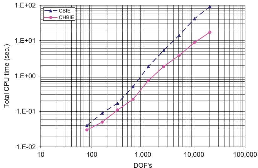
Fig. 6. Total CPU time used for solving the rotating cylinder problem by the fast multipole BEM with CBIE and CHBIE (log–log scale).
