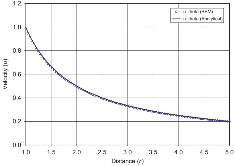
Fig. 5. Velocity  $u_\theta$  computed at points inside the fluid domain  $V$  (with 40 elements).
