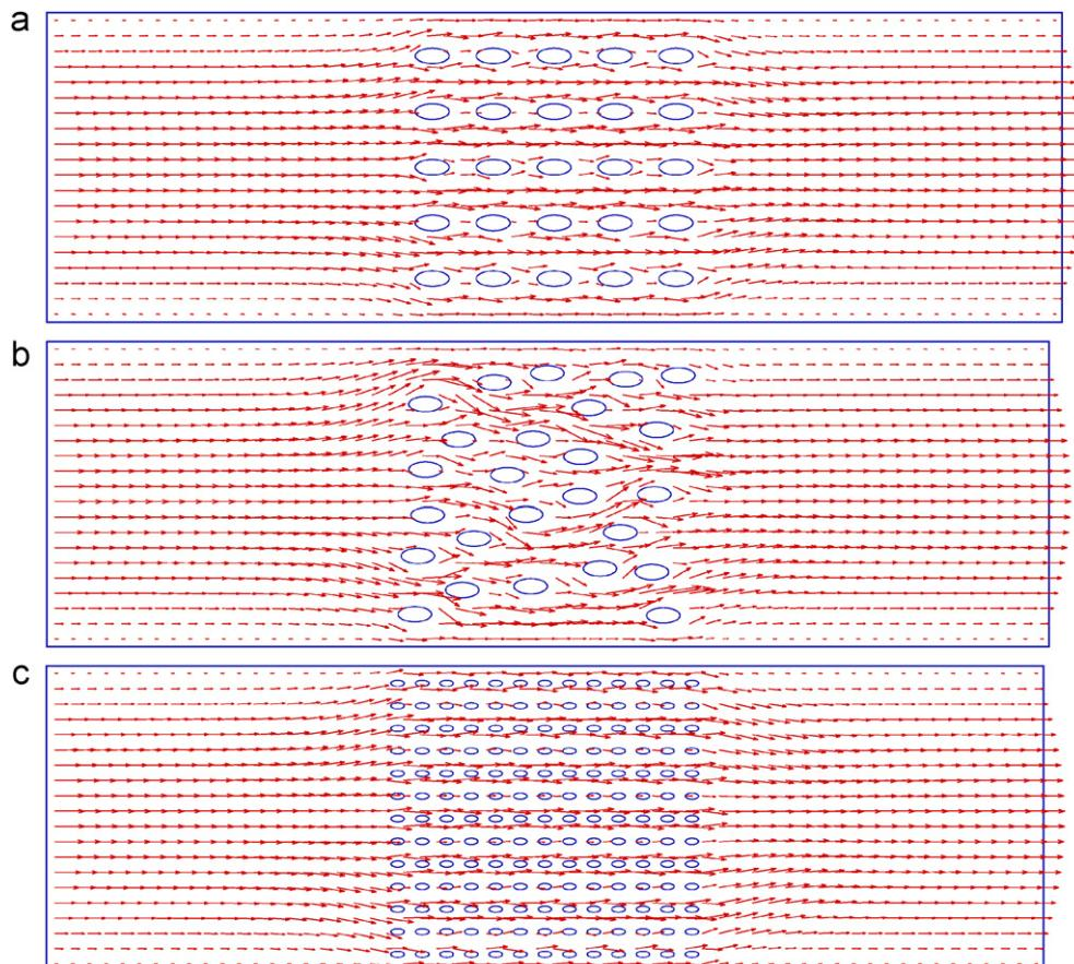
Fig. 10. Various BEM models of the channel with many elliptic cylinders ( $L = 3h$ ).
