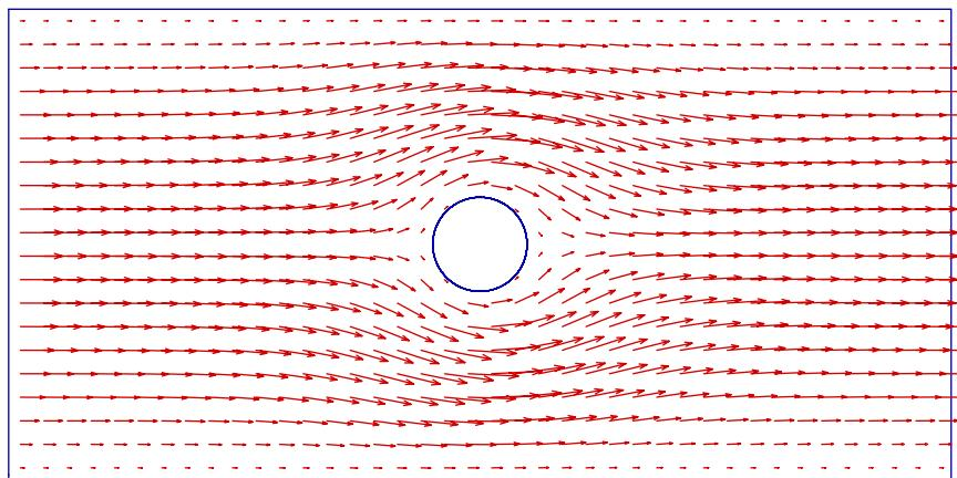
Fig. 9. Vector plot of the velocity field for one circular cylinder with  $a = 0.1h$  and  $L = 2h$ .
