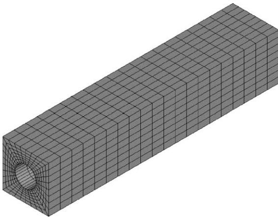
Fig. 5. A 3-D FEM model for the square RVE with a long CNT (CNT thickness = 0.4 nm, with one layer of elements).
