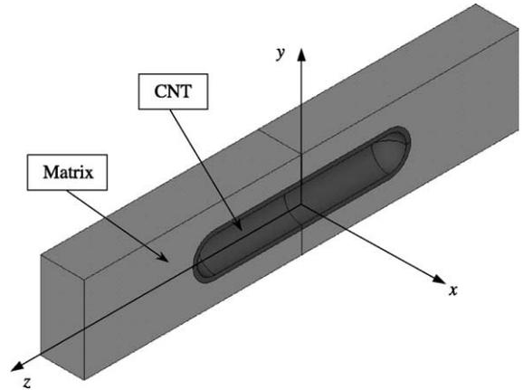
Fig. 2. A square RVE containing a short CNT shown in a cut-through view.
