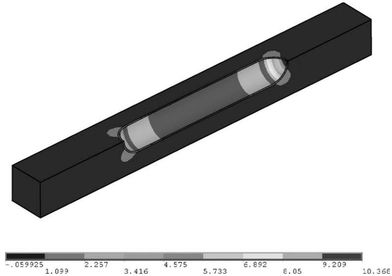
Fig. 9. Plot of the first principal stresses ( $\times \Delta L$ ) for the 3-D RVE under the axial stretch  $\Delta L$  ( $E^t/E^m = 10$ ).
