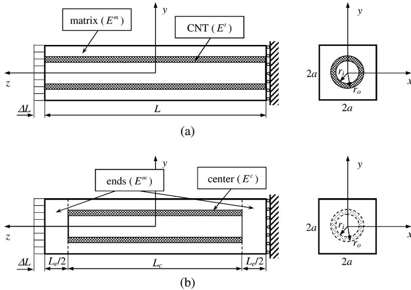
Fig. 4. Simplified strength of materials models based on the square RVEs for estimating the effective Young's modulus  $E_z$  in the CNT direction. (a) CNT through the length of the RVE; and (b) CNT inside the RVE ( $L = L_c + L_e$ ).
