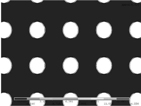
Fig. 7. Plot of the first principal stresses ( $\times p$ ) for the  $10 \times 10$  RVE model under lateral loading (zoomed in view;  $E^l/E^m = 10$ ).
