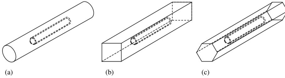
Fig. 1. Three possible RVEs for the analysis of CNT-based nanocomposites [7]. (a) Cylindrical RVE; (b) square RVE; and (c) hexagonal RVE.
