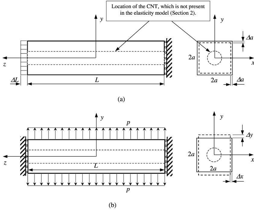
Fig. 3. Two loading cases for the square RVE used to evaluate the effective material properties of the CNT-based composites. (a) Under axial stretch  $\Delta L$ ; and (b) under lateral uniform load  $p$ .
