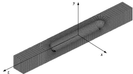
Fig. 8. A 3-D quarter-symmetry FEM model for the square RVE with a short CNT (CNT thickness = 0.4 nm, with one layer of elements).
