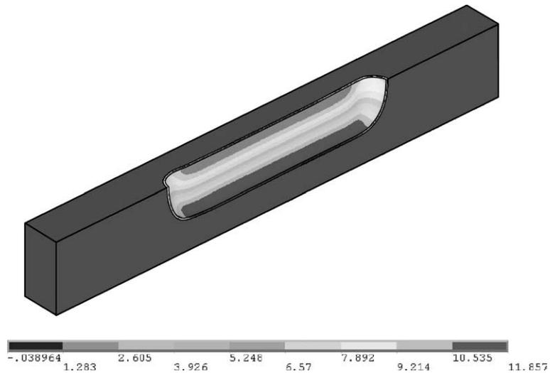
Fig. 10. Plot of the first principal stresses ( $\times p$ ) for the 3-D RVE under the lateral load  $p$  ( $E^t/E^m = 10$ ).
