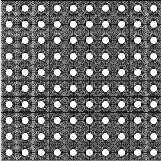
Fig. 6. A 2-D (plane strain) FEM model of the RVE containing  $10 \times 10$  long CNTs (CNT thickness = 0.4 nm, with one layer of elements).
