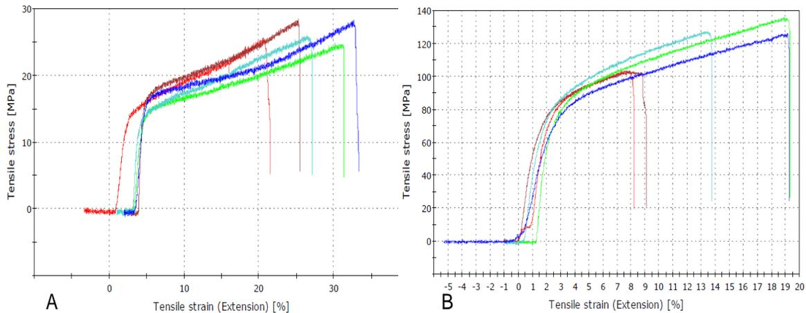
Figure 6. Tensile test results: A) for pristine CNT sheet; B) for post-processed CNT sheet.
