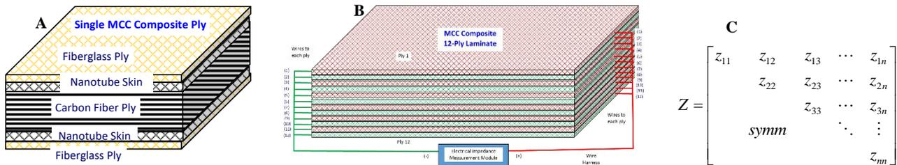
Figure 10. Construction of SW: (a) single ply SW; (b) a 12 ply SW laminate with 12 electrical circuits. The structure becomes the wiring harness and wires; (c) The electrical impedance will be modeled.
