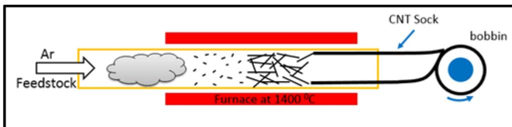
Figure 1. Schematic of catalyst floating manufacturing of CNT sheet.
