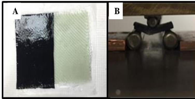
Figure 7. Composite strength testing: A) Fiberglass ply and CNT sheet lay-up; B) Short beam shear test.
