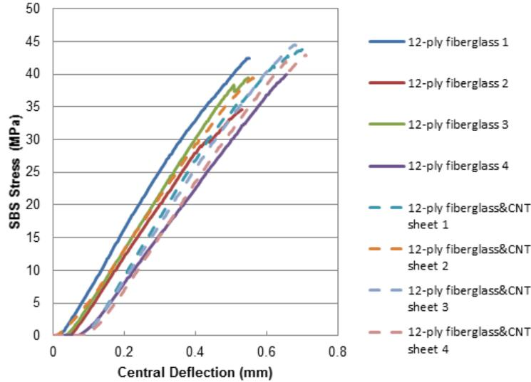
Figure 8. SBS results for 12-ply fiberglass composites with/without CNT sheet reinforcement.
