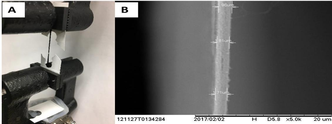
Figure 5. Tensile testing set-up: A) CNT Sheet test samples attached to test frame; B) Thickness of CNT sheet is about 1-2 microns.
