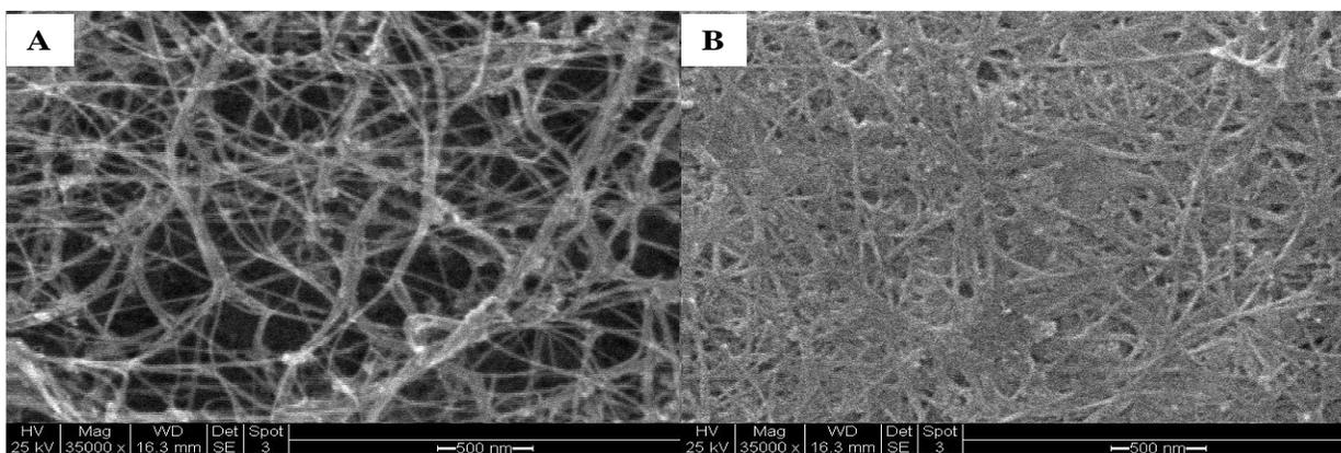
Figure 4. SEM image of CNT sheet: A) As produced; B) Pressure densified CNT sheet.
