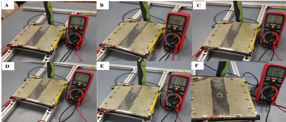
Figure 9. Increase in resistance of the structure with increase in impact energy: A) Impact energy 0.67 J; B) Impact energy 1.69 J; C) Impact energy 3.38 J; D) Impact energy 4.75 J; E) Impact energy 6.77 J; F) Impact energy 23 J.
