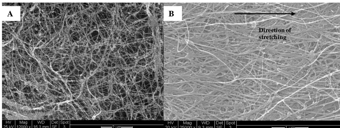
Figure 3. SEM image of CNT sheet: A) As produced; B) Stretched CNT sheet.
