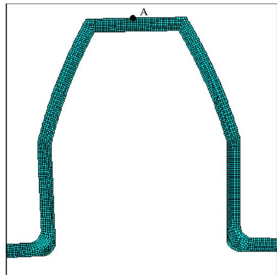
**Fig. 9** FEM mesh for the coating on one tooth of the gear model
