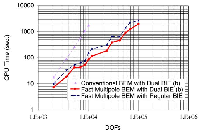
Fig. 9. CPU time for the conventional BEM and fast multipole BEM.
