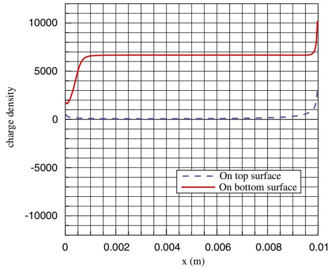
Fig. 8. Computed charge densities on the top beam surfaces (Fig. 6).
