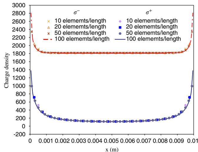
Fig. 3. Convergence of the BEM results using dual BIE (b) on the top beam in the parallel beam model ( $\epsilon = 1$ ,  $L = 0.01$  m,  $h = 0.0001$  m,  $g = 0.0011$  m,  $d = 0$ ,  $V = 1$ ,  $C = 0$ ).
