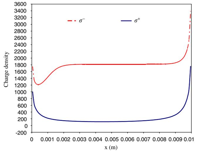
Fig. 4. Charge density on the top beam in the parallel beam model with offset ( $\epsilon = 1$ ,  $L = 0.01$  m,  $h = 0.0001$  m,  $g = 0.0011$  m,  $d = g$ ,  $V = 1$ ,  $C = 0$ , 210 elements per beam).
