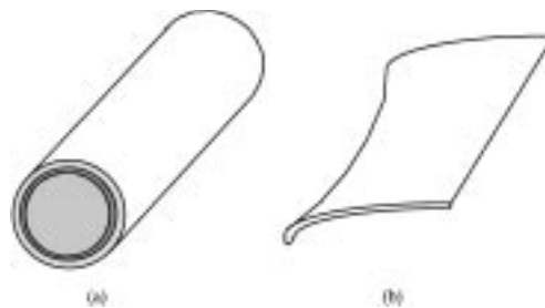
Figure 15. Shell-like structures: (a) layered structure; (b) thin structure with varying thickness (a blade)
